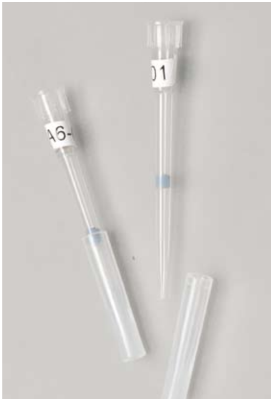
Left: Assembled SCAP PLS system sample cartridge Right: Numbered SCAP PLS system tip and cap
