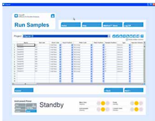
Fig. 3. Cliquid® mass spectrometer control software. Upon completion of the automated sample preparation method, a worklist file containing sample properties was automatically created, and this was uploaded into the Cliquid® mass spectrometer control software.
