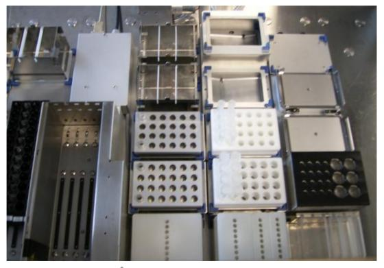
Fig 3: CyBi<sup>®</sup>-RoboSpense deck layout for peptide mapping
