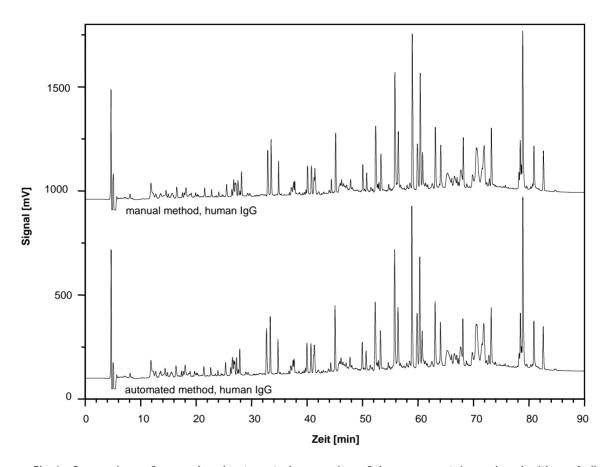
Fig 4: Comparison of manual and automated processing of the same protein analyzed with an Agilent HPLC system.
