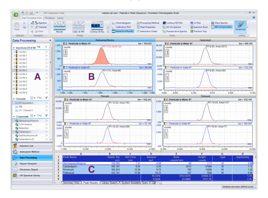
Detection parameters and component settings (Figure 5) in the Processing Method are applied to all component traces.
