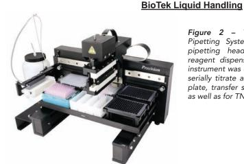
Figure 2 – The Precision<sup>™</sup> Microplate Pipetting System combines an 8-channel pipetting head and an 8-channel bulk reagent dispenser in one instrument. The instrument was used to dispense U937 cells. serially titrate antibody across a 96-well PP plate, transfer samples from plate to plate, as well as for TNF $\alpha$  and reagent dispensing.
