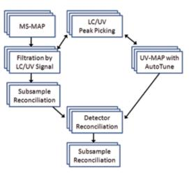
Figure 4. Schematics of automated data process (ADP) developed based on AutoChrom to integrate and track chromatography peaks for QbD experimentation reports.
