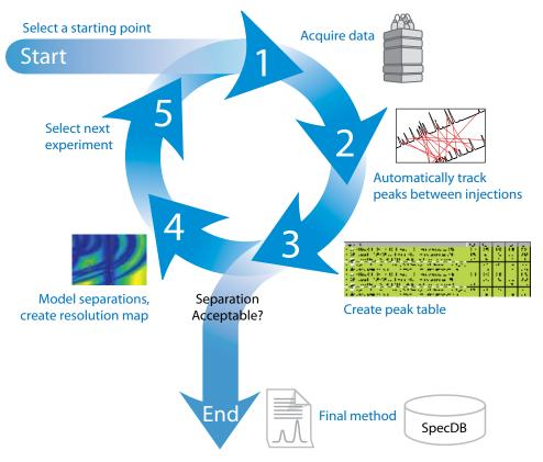
Figure 3. Automated execution of QbD RPLC method development with AutoChrom and Empower.
