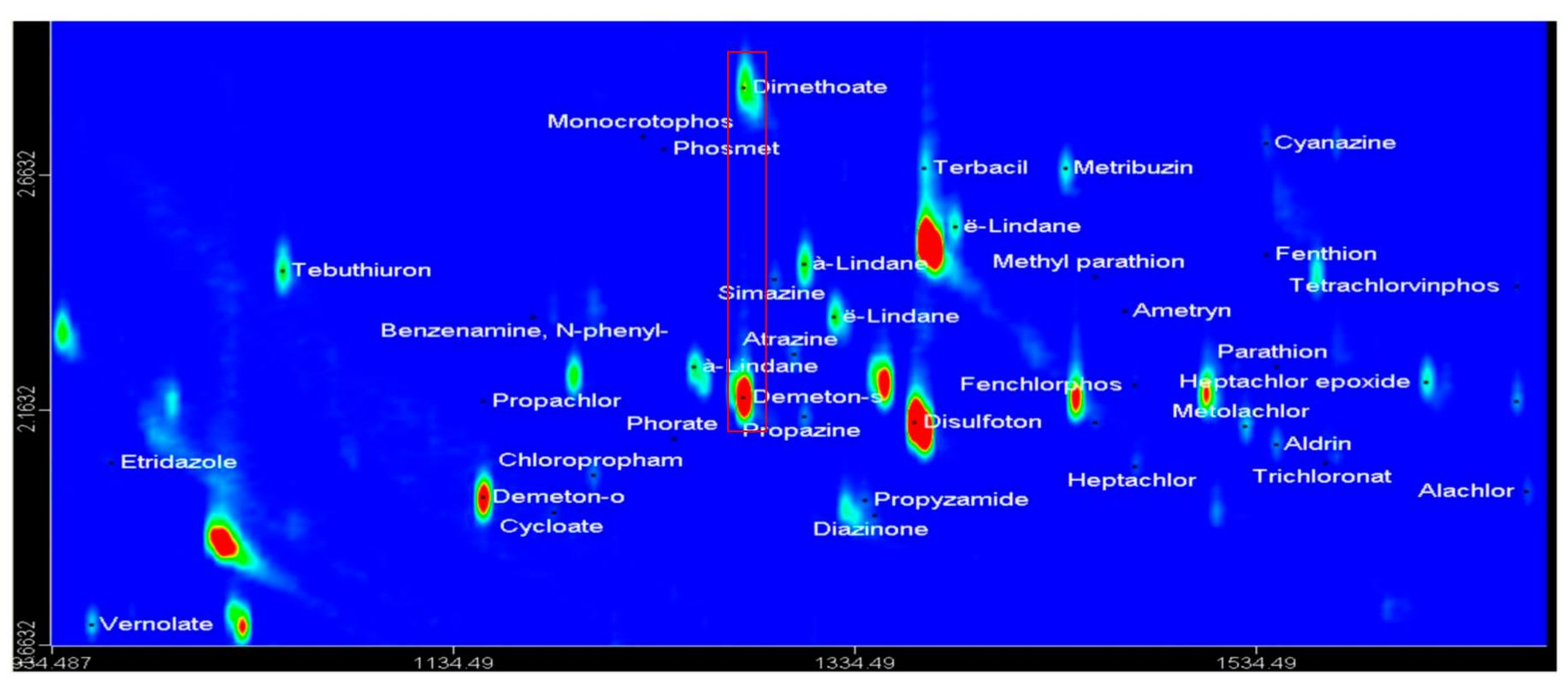
Figure 6. A portion of the LECO Pegasus 4D GCxGC total ion contour plot highlighting the region in which pesticides would have coeluted in a traditional one-dimensional GC analysis. The value of second-dimension GCxGC separation is evident in this figure.
