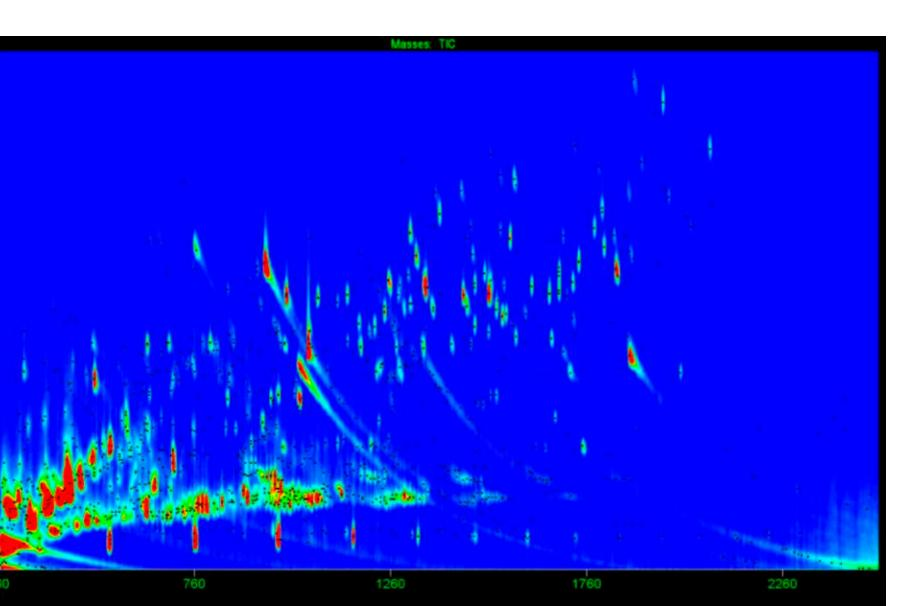
Figure 3. The total ion contour plot for the pesticide spiked QuEChERS extract of blueberry jam commodity.
