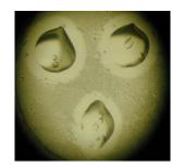
mosquito can multi-aspirate and accurately dispense three different drops into each well of a 96-well hanging drop screen.
