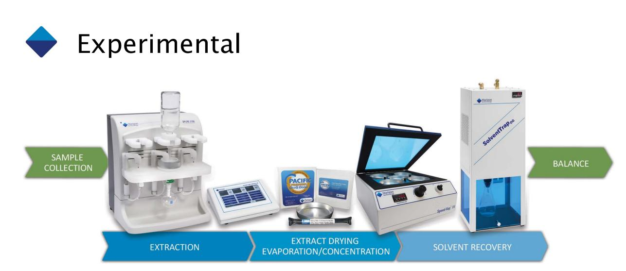
The evaluation was performed using the SPE–DEX 3100 Oil & Grease Extraction System (Horizon Technology, Inc.). The SPE–DEX 3100 system was set up with the larger disk holder (100 mm). The evaporation step, prior to gravimetric measurement was performed using the Speed–Vap<sup>®</sup> IV evaporation system with the 5-position rack and 105-mm aluminum weighing pans (Horizon Technology, Inc.). Pacific<sup>™</sup> Premium solid phase extraction disks were used for this work (Horizon
