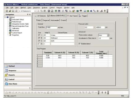
Figure 2: Typical OpenLAB client screen for instrument control. More than 300 different instruments from a variety of different instrument vendors can be controlled within OpenLAB though a uniform software interface.
