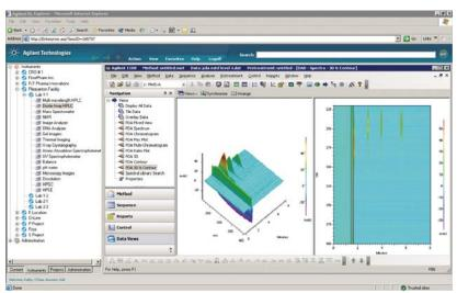
Figure 1: Typical OpenLAB provides both an "instrument" view of the enterprise as well as a "content" view. In this example, an authorized user has accessed the main OpenLAB instrument view. Instruments can be located in the convenient OpenLAB left pane in the hierarchy of "LOCATION / CABINET / DRAWER / FOLDER" so that instruments can be easily assigned into a project or location folder.
