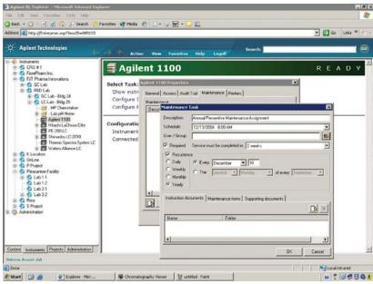
Figure 5: OpenLAB instrument maintenance setup screens allow creation of maintenance tasks including links with other documents (instructions, checklists, etc.) managed by the OpenLAB Enterprise Content Manager. If desired, instruments can be managed by OpenLAB such that the scheduled maintenance must be performed or the instrument cannot be run by users.
