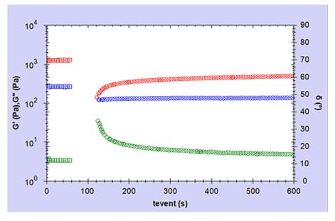
Figure 1 – Step strain/shear rate curves for a toothpaste (Elastic Modulus G' in red; Viscous Modulus G' in blue; phase angle  $\delta$  in green)
