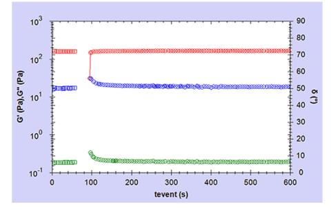
Figure 2 – Step strain/shear rate curves for a hair gel (Elastic Modulus G' in red; Viscous Modulus G'' in blue; phase angle  $\delta$  in green)
