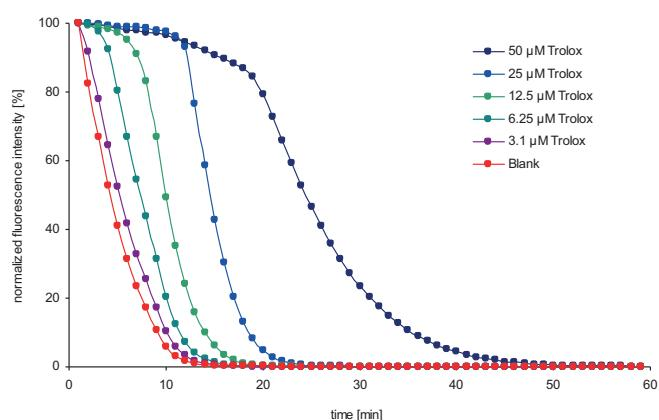
Figure 1 Signal curves measured for different Trolox concentrations (results normalized to initial fluorescence signals after AAPH addition).
