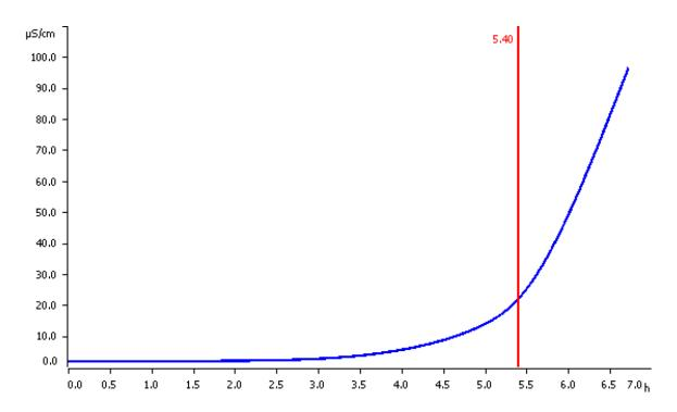
Determination of the oxidation stability of corn oil using the Rancimat method.
