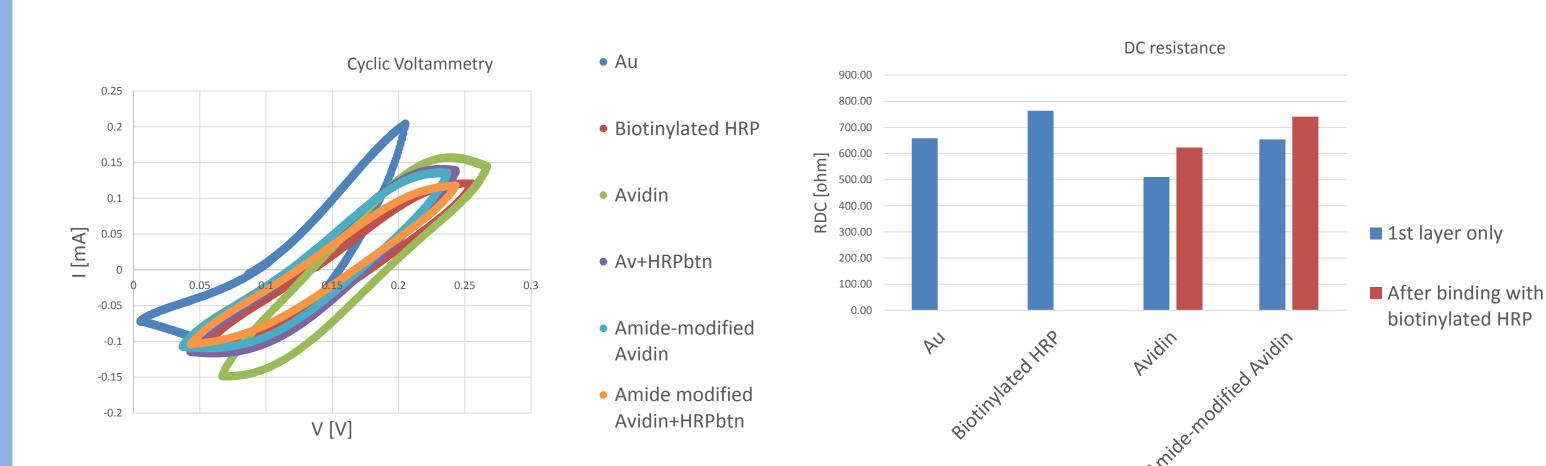
Fig. 4: Total resistance ( $R_e + R_{e,p} + R_{ct}$ ) calculated for different protein configurations
