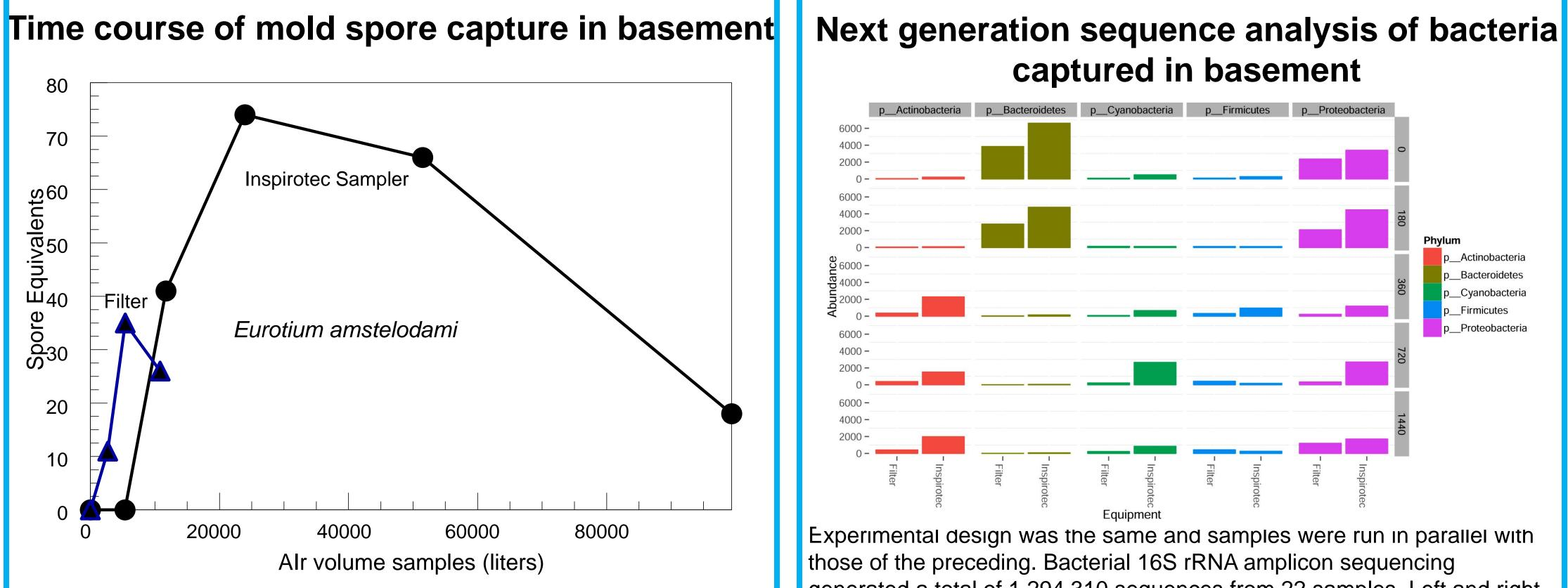
Five Inspirotec samplers and 3 filters with pumps were run in parallel in the basement as in the preceding table, and removed for analysis at timed intervals up to 24 hrs. The results are plotted as volume of air sampled during the time interval. Amounts are number of spore equivalents captured per sample. For both, the spore equivalents determined by qPCR became detectable at 6 hrs of sampling.
