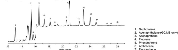
Figure 3. Soybean Oil Extract, 10 ng/g Spiked: GC/MS-SIM Analysis
