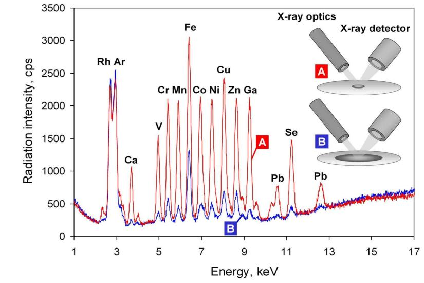
EDXRF spectra of two reference samples containing 0.5 µg of each element. Samples A and B of various diameters (ca. 1 and 5 mm, respectively) deposited onto the Millipore filter are excited with an X-ray beam of 900 µm focus spot size.
