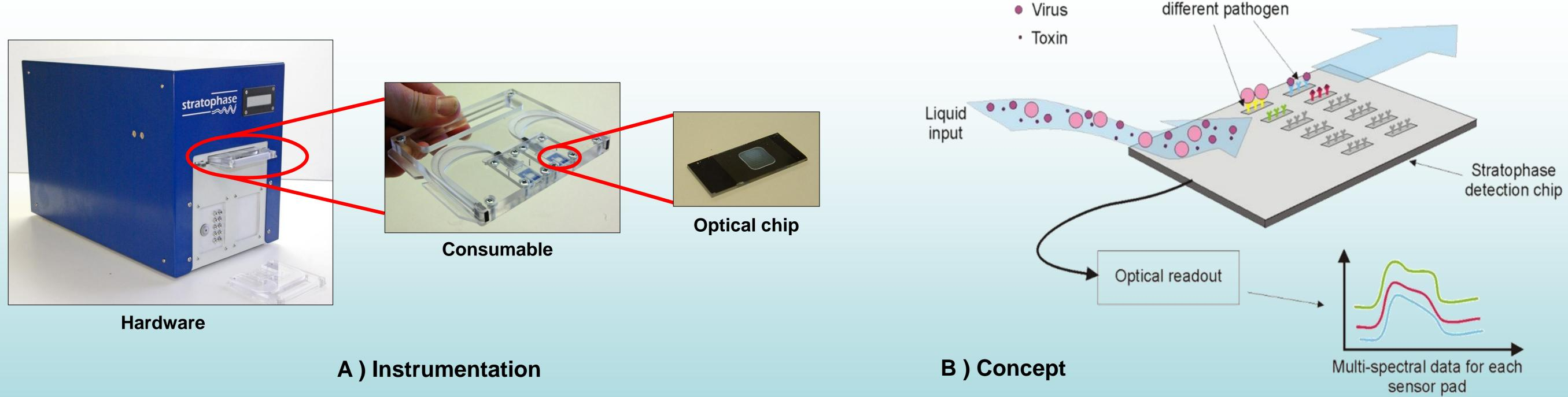
Figure 1: SpectroSens Technology A). SpectroSens detector with plastic plug-in consumable comprising two multi-channel optical sensor chips [1]. B) Schematic illustration of the principles of SpectroSens biological detection: target pathogens in the liquid sample are captured by specific antibodies immobilised on individual sensing channels within the optical sensor chip. Changes in optical spectra associated with selective pathogen binding are captured by the SpectroSens detector<sup>[2]</sup>.
