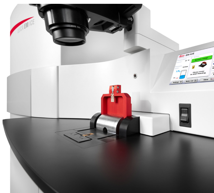
Fig.3. Assembly of two half cylinders and a middle plate/PCB for electrical stimulation in the Leica EM ICE
