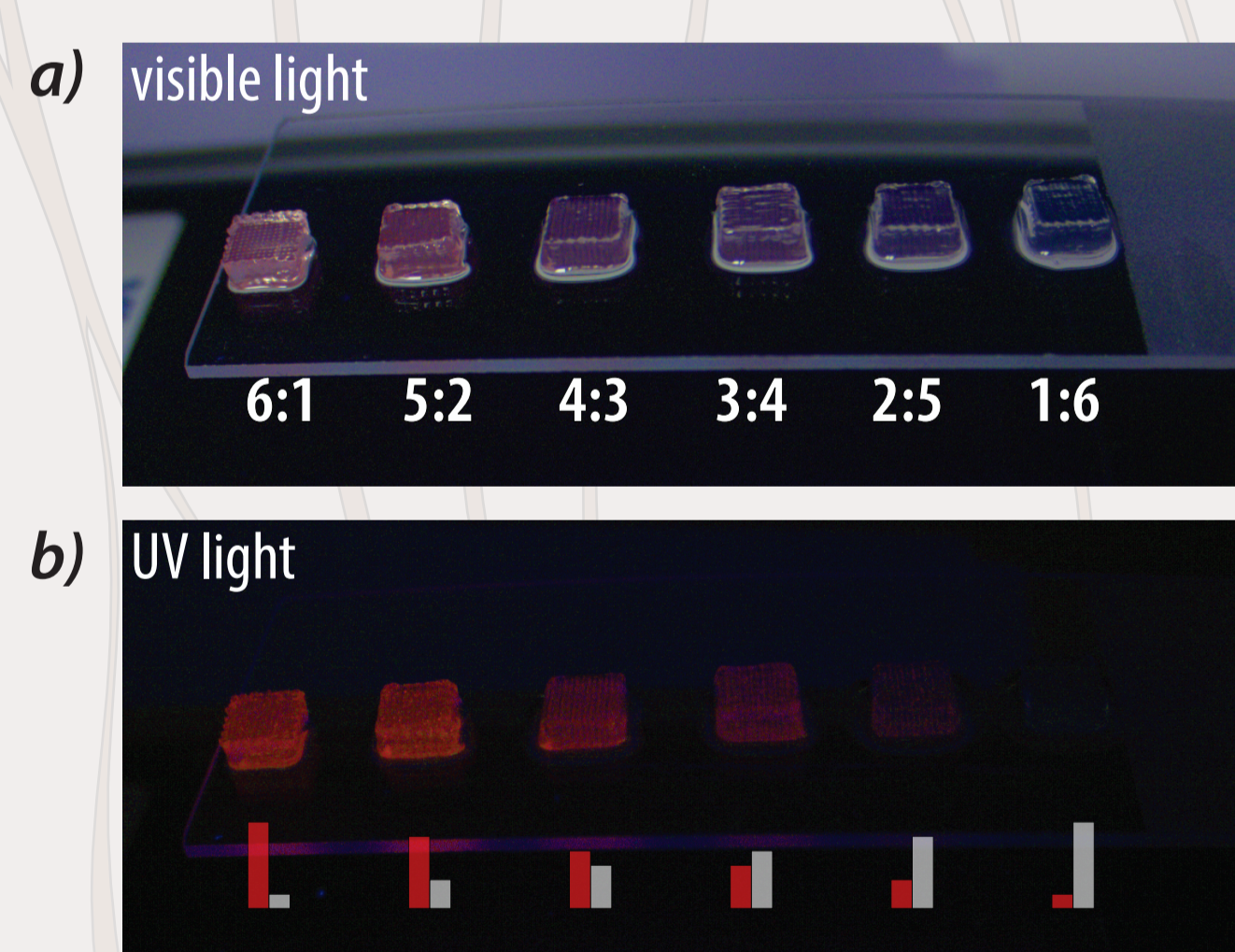
Figure 4: Magnified photographs of 3D printed constructs obtained using a micro-mixing microfluidic device in line with the extruder. Two hydrogel-precursor solutions, one loaded with red fluorescent beads, were mixed at different proportions inside the microfluidic chip. The ratio between fluorescent and non-fluorescent ink was changed for each construct as reported in figure. The constructs were all produced in a single printing experiment. a) Constructs illuminated with ambient light; b) constructs illuminated with UV light.
