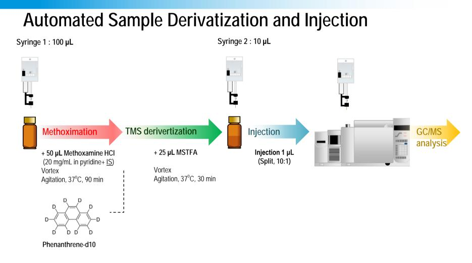
"Just -in-Time" derivatization and injection to GC-MS
