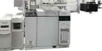
Agilent GC-MS system 7980A-5975C with PAL RTC
