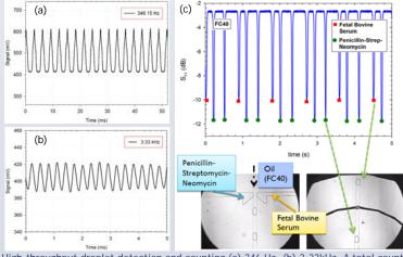
High-throughput droplet detection and counting (a) 346 Hz, (b) 3.33kHz. A total count of 2 million droplets was counted in ten minutes without missing any droplets. (c) Showing label-free content sensing of individual droplets; the coordinated optical imaging and microwave sensing results for Fetal Bovine Serum and Penicillin antibiotic mixture droplets. Conclusion
