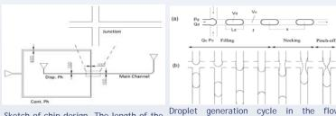
Sketch of chip design. The length of the main channel was set to be 2.5cm
