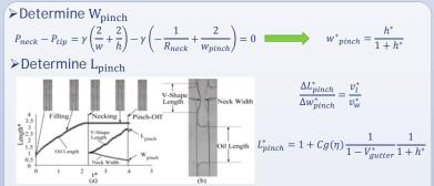
Variations of V-shape length, neck width and oil length during a droplet formation cycle
