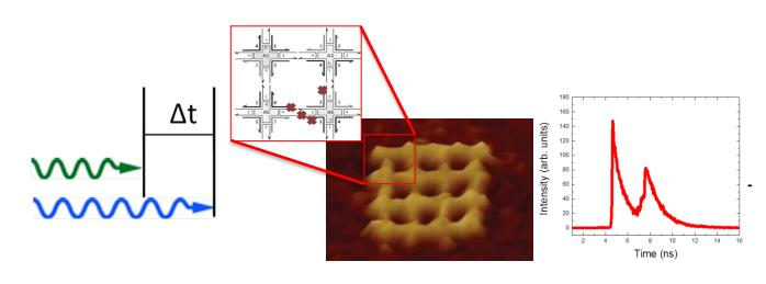
Input Laser Pulses FRET Network > Fluorescence Output
