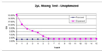
Figure **5**. The unoptimized mixing protocol at 2200 RPM takes around 8 minutes before consistent %CV values are reached.
