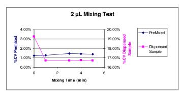
**Figure 7.** Control wells show consistent %CV values for all measurements, corresponding to the left y-axis. Test wells show consistent %CV values after 1 minute of mixing at 2600 RPM corresponding to the right y-axis.
