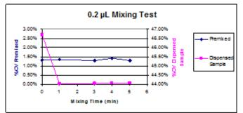
**Figure 9.** Control wells show consistent %CV values for all measurements, corresponding to the left y-axis. Test wells show consistent %CV values after 1 minute of mixing at 2600 RPM corresponding to the right y-axis.
