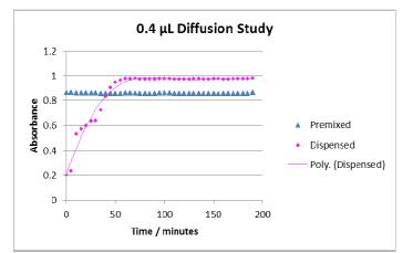
**Figure 2.** Diffusional mixing of 0.4  $\mu$ L Range E solution into 200  $\mu$ L of Diluent in a 96-well microplate takes more than 90 minutes before a homogenous mixture is achieved.
