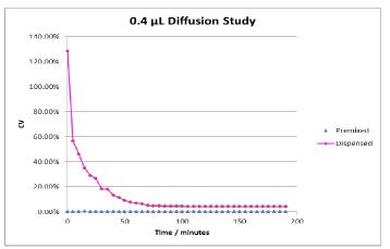
Figure 3. Diffusional mixing of 0.4  $\mu$ L Range E solution into 200  $\mu$ L of Diluent.
