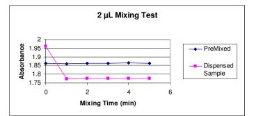
**Figure 6.** Mixing of the 2  $\mu$ L sample in 53  $\mu$ L of Diluent was achieved in 1 minute as illustrated by the consistent %CV values recorded after the initial, unmixed absorbance measurement. The mixing cycle duration was 60 seconds for each trial and speed was 2600 RPM. Control wells show consistent absorbance values for all measurements, as expected.
