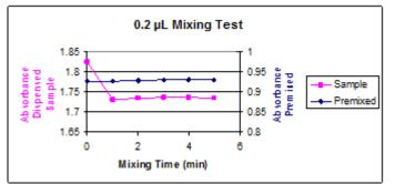
**Figure 8.** Mixing efficiency of the 0.2  $\mu$ L sample is indicated after 1 minute of mixing at 2600 RPM by the consistent absorbance measurements after the initial measurement.
