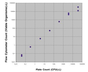
**Figure 6** Correlation between the concentration of *B. globigii* determined by flow cytometry and by plating on BD Trypticase Soy Agar
