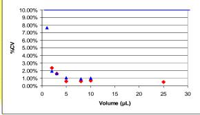
**Figure 1.** Comparison of precision (%CV) of Direct and Over-aspiration methods using the MVS. Volumes included in the graph are actual volumes delivered as opposed to target volume requested by the RapidPlate.
