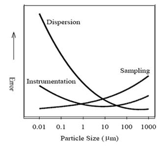
Figure 1: Sources of error as a function of particle size in laser diffraction [1].
