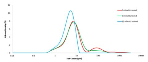
Figure 2: Particle size distributions from fine grade lactose measured with 0, 5 and 10 minute applications of ultrasound.
