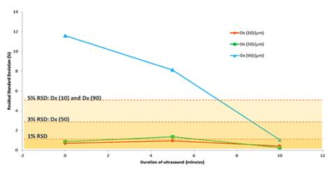
Figure 3: Relative standard deviation, %, vs duration of ultrasound, minutes. The measurement repeatability is less than 1% for the Dv10m Dv50 and Dv90 once the sample is fully dispersed.
