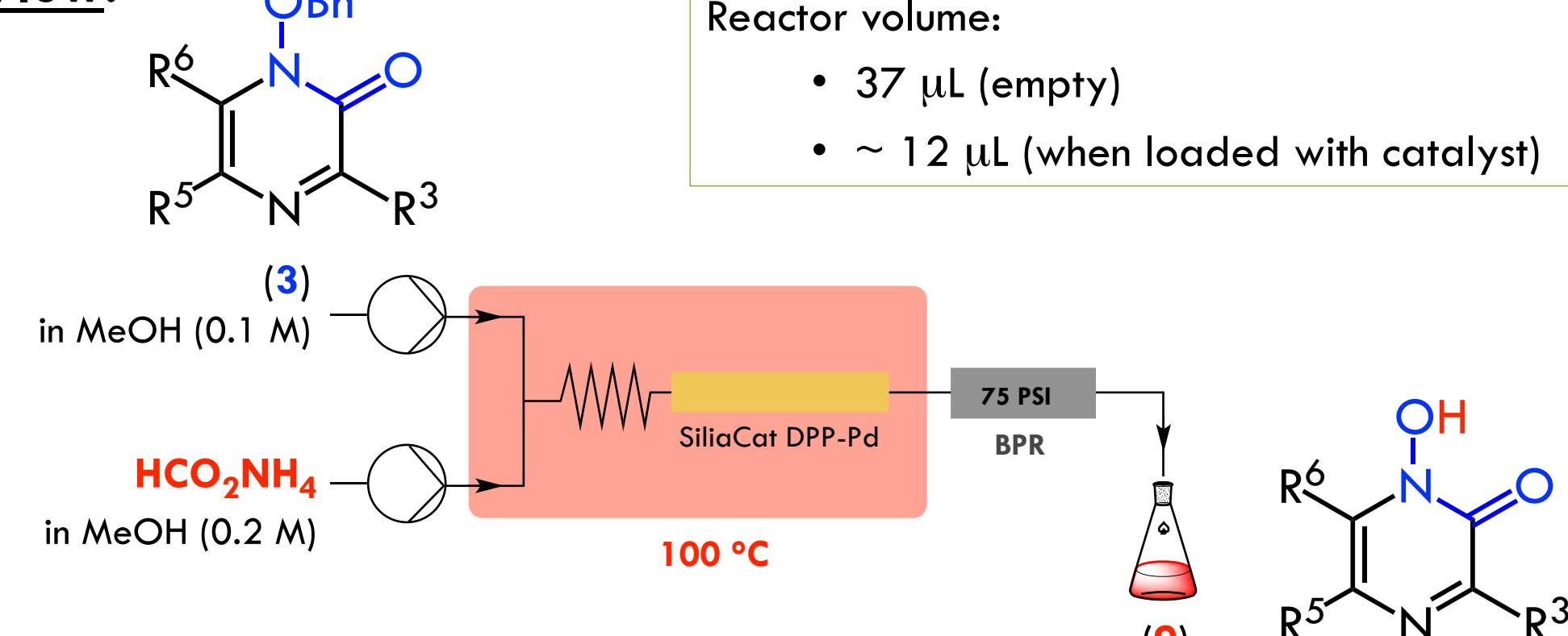
Conditions: (3) (0.1 mmol, 1 equiv., 0.1 M), SiliaCat®DPP-Pd (0.8 mol%), HCO<sub>2</sub>NH<sub>4</sub> (0.2 mmol, 2 equiv., 0.2 M).
