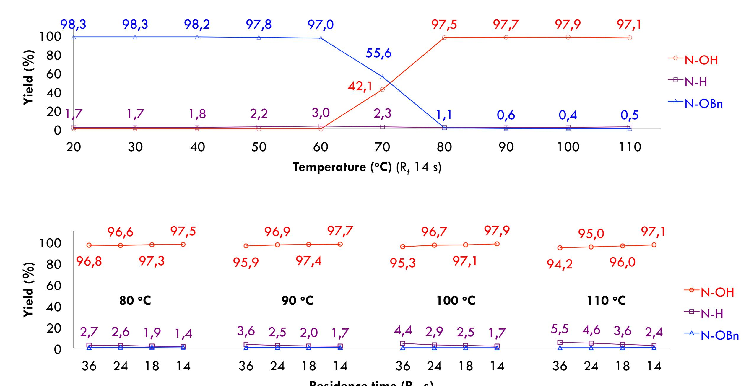
★ The ideal flow conditions for debenzylation of O-benzyl precursors: HCO<sub>2</sub>NH<sub>4</sub> as hydrogen donor, SiliaCat® DPP-Pd as catalyst, reaction temperature above 100 °C and residence time of 14 s. These conditions were applied to synthesise other N-hydroxypyrazinones (**9a-x**).
