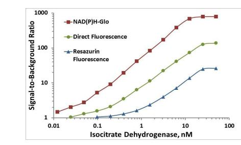
NAD(P)H-Glo Detection System – measure changes in reduced forms in the presence of oxidized forms
