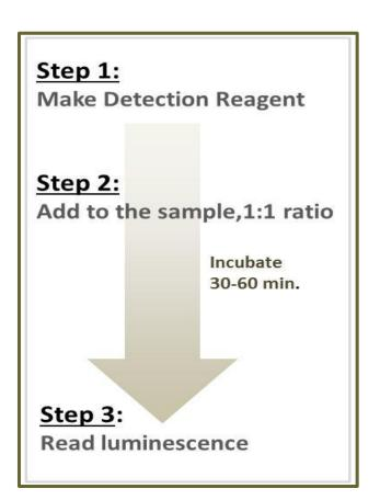
✓ Assay sensitivity enables detection of total NAD+NADH or NADP+NADPH directly in 96/384wells
