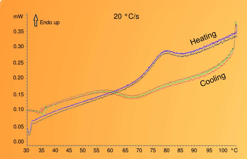
Measurements of a 10 % lysozyme-in-water solution.
