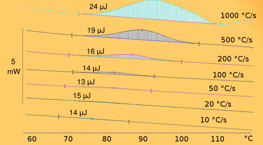
Heating curves of a 10 % lysozyme-inwater solution measured at scan rates between 10 °C/s and 1000 °C/s. As expected the protein-unfolding peak becomes bigger at higher scan rates, and shifts to higher temperatures. The chip gap size is about 30 µm.
