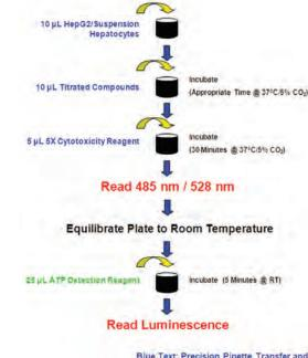
Blue Text: Precision Pipette Transfer and Dispensing Red Text: Synergy H4 Microplate Reads
