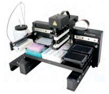
Figure 1 – Precision<sup>™</sup> Microplate Pipetting System combines an 8-channel pipetting head and an 8-channel bulk reagent dispenser in one instrument. The instrument was used to perform the serial dilutions of test antibodies and binding proteins, and transfer aliquots into the LV384-well assay plates.
