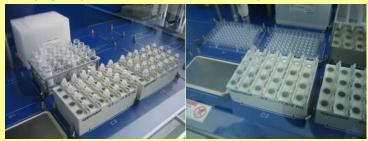
Figure 4. The samples are delivered from the Chemspeed automated synthesis platforms and placed directly onto the deck of an Eppendorf epMotion 5075LH liquid handling platform where the centrifuged samples are rapidly prepared and processed. This purification process is over 50 times faster than traditional manual methods and is scalable up to 100ml allowing researchers to rapidly produce fully characterised libraries of functionally diverse polymer latexes as shown in figures 4 and 5
