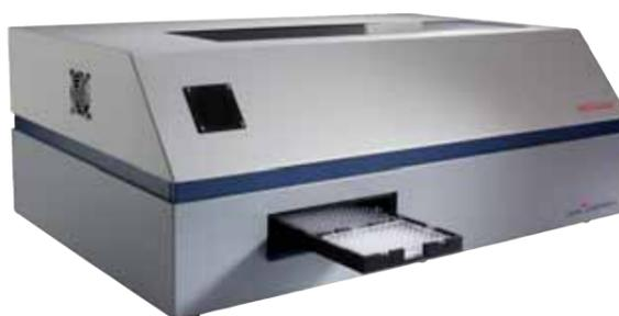
Fig. 4: BMG LABTECH's NOVOstar with unique pipetting system allows for instantaneous reading upon agonist stimulation.
