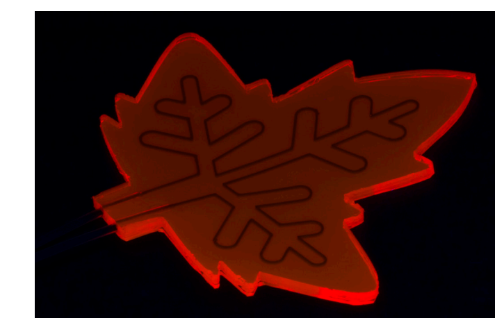
3D-model of the standard device and photograph of a leaf-shaped LSC-PM.
