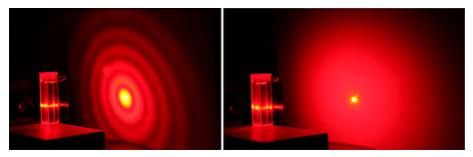
Figure 3: Diffraction patterns for a 5 µm sample (left) and an 800 nm sample (right) show how the light scattering pattern produced by a sample is strongly influenced by the size of particles within it. (Source: Kevin Powers, PERC, University of Florida)
