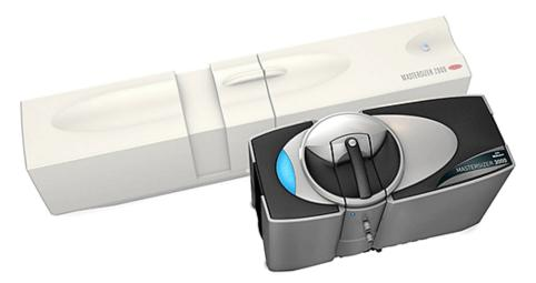
Figure 7: Mastersizer 2000 with its successor, the Mastersizer 3000. A systematic 'QbD' approach allowed designers to increase measurement range while at the same time decreasing the footprint of the optical bench.
