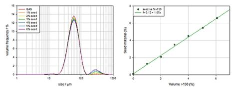
Figure 8: Bimodal distribution of glass beads undergoing wet measurement to test the accuracy of the wet dispersion system.
