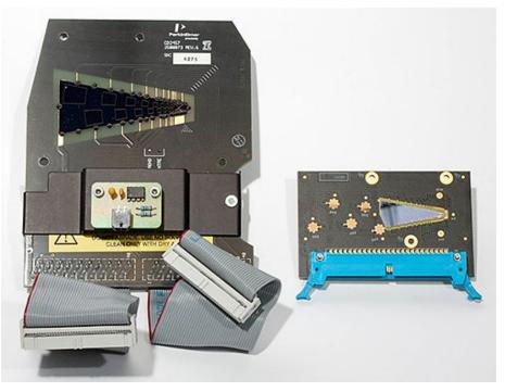
Figure 5: Comparing the size of the focal plan detector for the Mastersizer 2000 (left) with that of the Mastersizer 3000 (right) shows the size reduction that was achieved. Decreasing the detector size satisfies the requirement to shorten the optical bench and increase the upper particle size measurement range.
