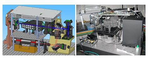
Figure 6: CAD drawn optical bench and x-model prototype. Theoretical and actual results showed good correlation.
