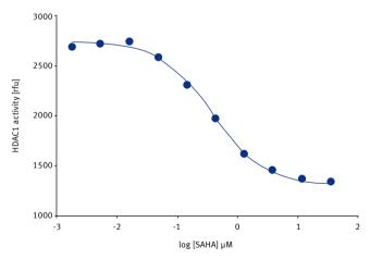
Fig. 4: IC<sub>50</sub> value of HDAC1 with SAHA. HDAC1 (4.5 nM) was incubated with 1:3 serial dilution of SAHA and 20 μM Boc-Lys(Ac)-AMC after performing a two-step activity assay by measuring the release of AMC (excitation filter: 340/10 nm; emission filter: 460/10 nm).
