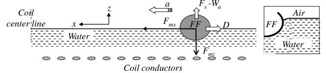
Magnetic force on ferrofluid droplet within the magnetic field :
