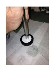
Fig.1: Reflectance : NIRS XDS SmartProbe Analyzer
