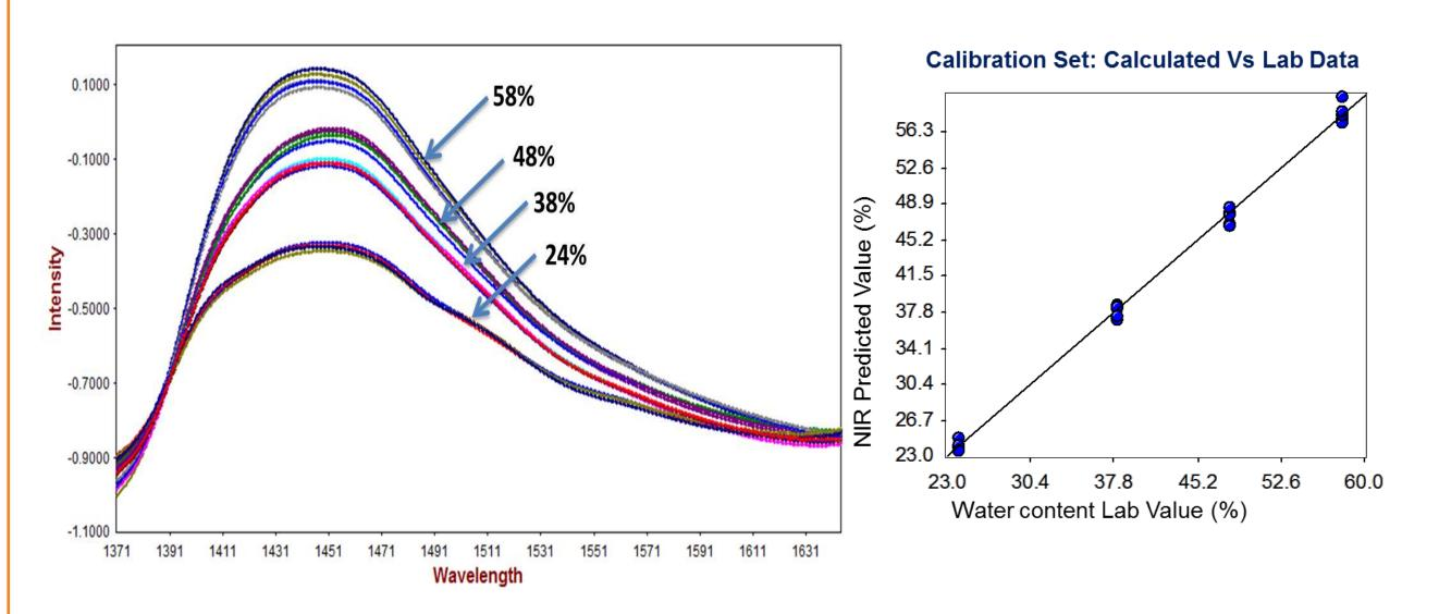
**Fig.5:** shows the water absorption region of the NIR absorption spectra of the contact lenses with various percentages of embedded water collected using RCA in trans-reflectance mode. The standard error of calibration using only two factors was 0.82 % with an  $R^2$  value of 0.9964.
