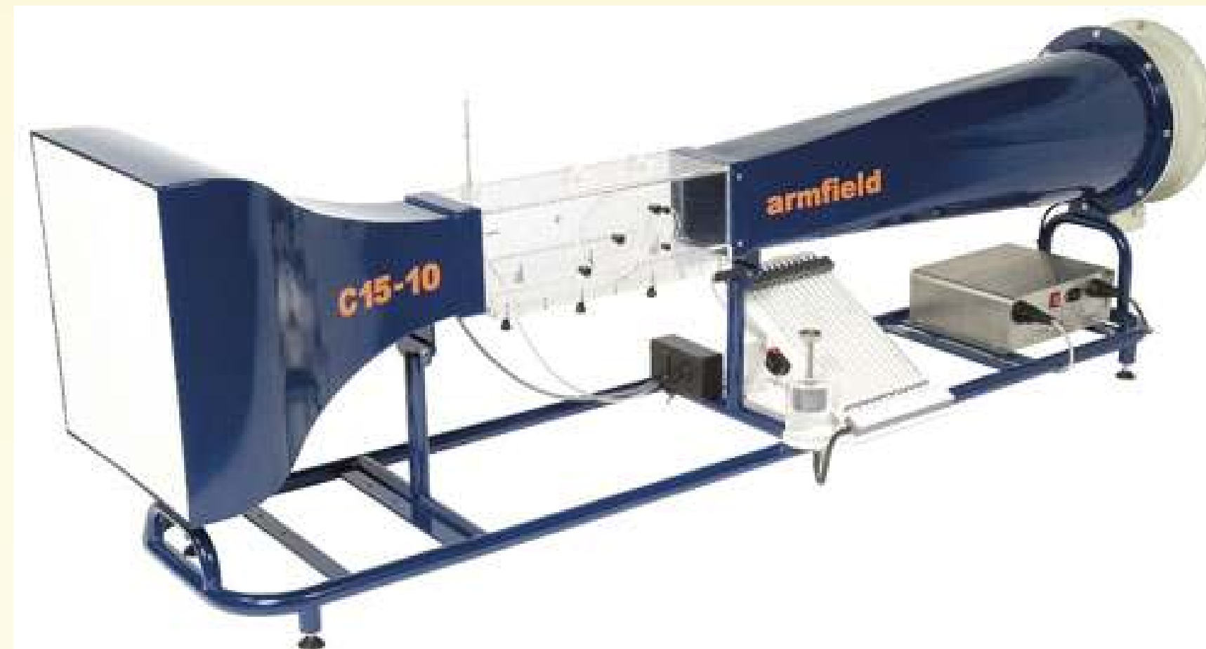
FIGURE 1: A small, benchtop wind tunnel, with visible working section (www.armfield.co.uk).
