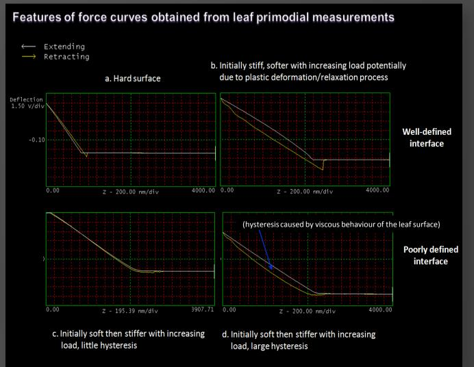
Differences in cell wall extensibility can be measured and mapped using AFM with great resolution showing spatial heterogeneity of extensibility at cellular and tissue levels.
