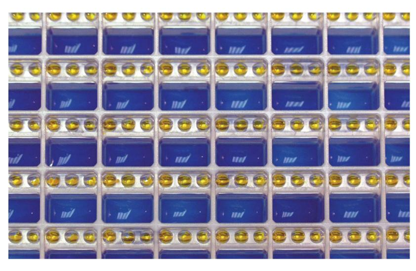
**Figure 5:** Actual photo of a Greiner 963 Crystallization plate with each main reservoir containing 80  $\mu$ l of blue dye solution and three different drop volumes of 10% Tartrazine dye solution on the three top shelves. The drop volume in each top shelf is 300 nl, 200 nl and 100 nl respectively. Drops were dispensed with the Honeybee 963 System.
