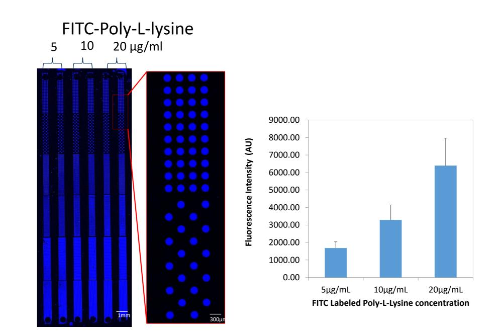
**ECM protein nanopaterning:** In order to test the uniformity of protein patterns, microscope slides were patterned with different concentrations of fluorescent-labeled ECM proteins using the InnoStamp 40 automate. A representative image for FITC-labeled poly-L-Lysine patterning is shown. Different 50-150  $\mu$ m patterns such as horizontal or vertical lines and dots were used as nanopaterns (pitch 40-220 $\mu$ m).
