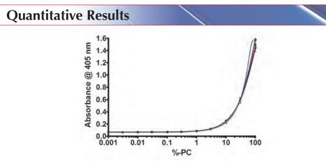
Figure 7 – Demonstration of Automated System to perform quantitative assays. Log dilutions of the Avioq HIV-1 positive control (PC) were assayed and the mean and standard deviation plotted for 4 separate assay plates. Each data point represents the mean of four wells.
