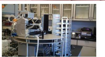
Figure 8 – Images of Modular Robotic Assay System. Photo depicts complete modular automated system with random access stacks, Mezzanine Table, 405 Touch Microplate Washer and MultiFlo Microplate Dispenser. The Eon Microplate Spectrophotometer (not seen) is located on other side of Orbitor RS plate mover
