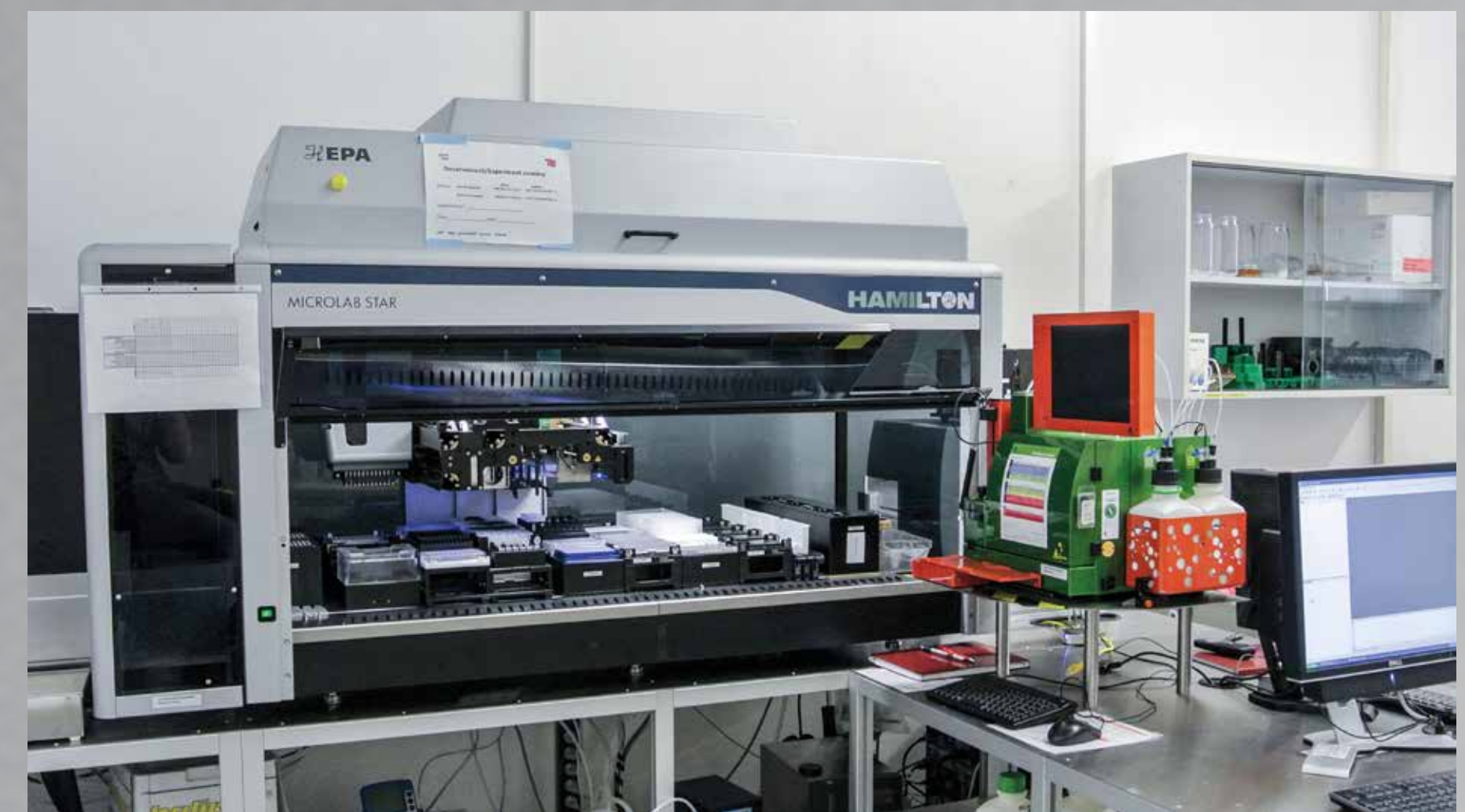
Laboratory of the AutoBio project partner TU Berlin where iLAB is used to collect experiment data running on different platforms: Hamilton Microlab Star with integrated Flow Cytometer (Miltenyi MACS-Quant Analyzer) and Spectrophotometer (Biotek Synergy MX)
