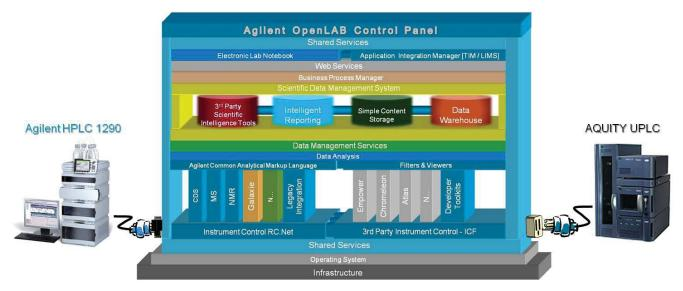
Figure 5 - OpenLAB Architectural Framework
