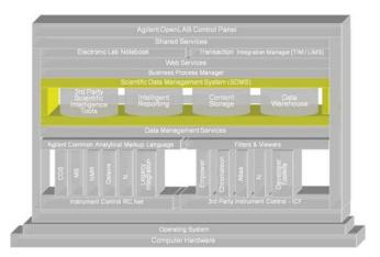
Figure 10 - OpenLAB Scientific Data Management System Component
