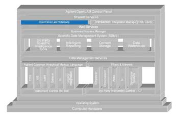
Figure 9 - OpenLAB Electronic Lab Notebook Architecture
