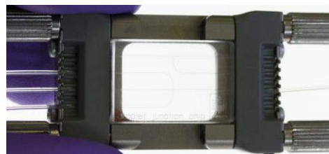
Image of droplet junction chip with H-interface, connectors, and tubing assembled. Channel depth is 100 \mu\text{m} ; fluid flow is from left to right.
