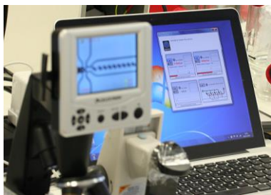
The educational system uses USB based PC control to change the pressure (and flow rates) in the fluidic system.
