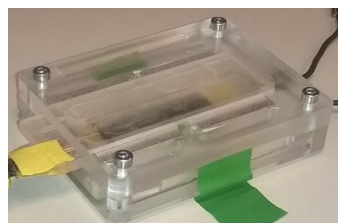
Fig. 2: An experimental setup with a heater prototype containing a mock-up of a microfluidic cartridge (75 mm x 25 mm). The NC milled PMMA structure contains a self-regulating resistive heating element and a temperature sensor for temperature recording.
