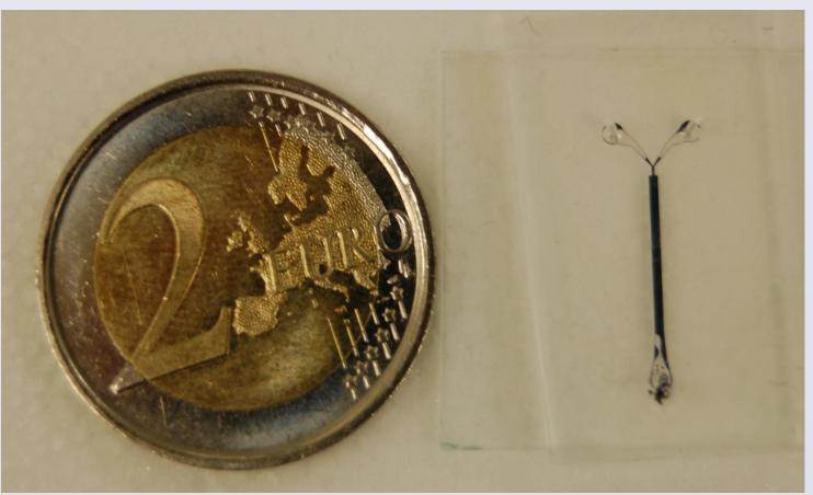
Lines and rectangular bases for femtosecond laser ablation were created using PDMS molds of SU-8 line structures. 10 wt% polystyrene in anisole is spin-coated at 4,500 RPM to achieve partial dewetting. The dewetted layer is stamped off at 170°C and low pressure (manual) and the inner layer is stamped at 170°C and high pressure (manual).
