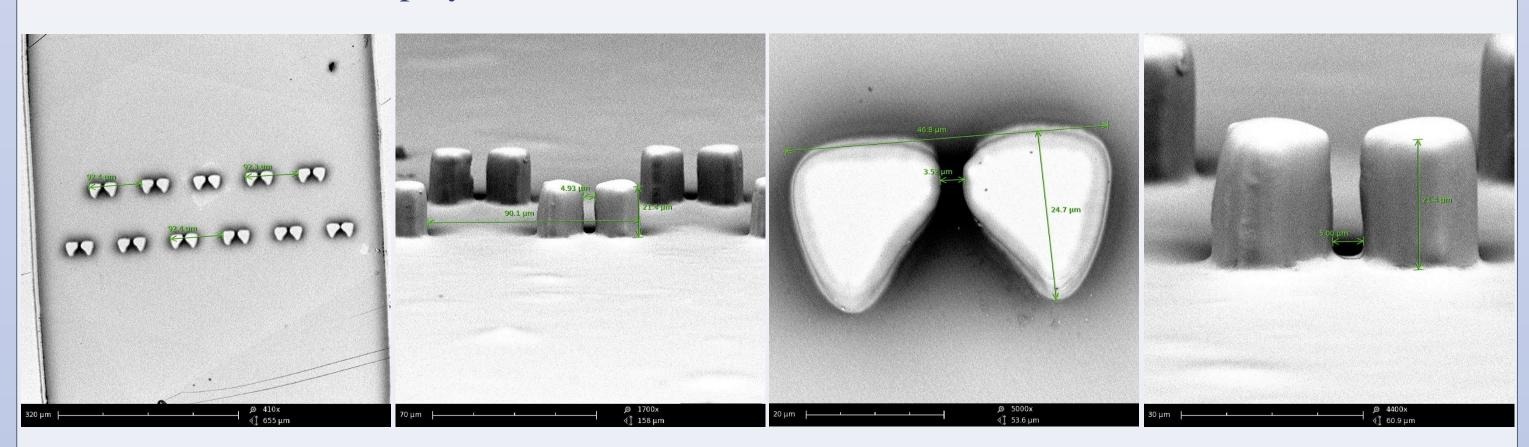
Polystyrene lines for guided 1D migration were fabricated using both spin-dewetting/stamping and femtosecond laser ablation. Stamping produced more consistent line heights and edges and did not produce debris as in ablation, but the pressure from stamping caused some lateral displacement which lead to slight misalignment with the traps. The debris from ablation may play a significant factor as cells typically prefer areas of higher surface energy for focal adhesion formation.
