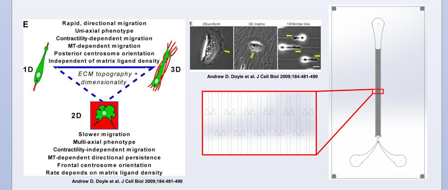
This device design will allow precise microfluidic assessment of potential drug targets to limit cancer cell migration due to its high cell seeding predictability and fluidic control.
